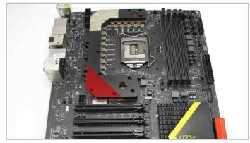
**6**. The board is now ready for use. When you first boot it is highly advisable to monitor chipset temperatures. If they appear high you may need to remove and refit the block. Finally you can place the optional XSPC badge on the position marked above in red.
