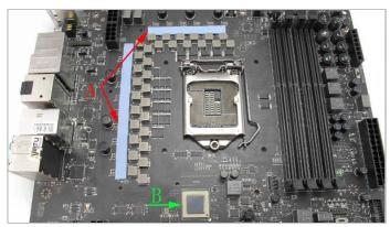
3. Remove the film from both sides and place the blue thermal pads on the positions marked A and the grey pad on the position marked B.
