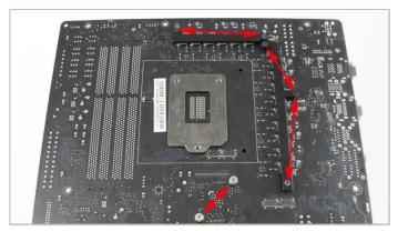
1. Turn the board over and remove the six screws highlighted above. Keep these to one side, they will be needed in step 5.
