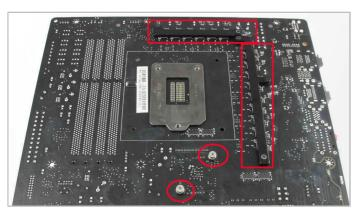
5. With one hand on the block, turn the board back over. Refit the two backplates using the original screws and fit the two screws below the backplates. You should gradually tighten them in turn so even pressure is applied.
