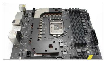
4. Remove the plastic film from the water block and carefully place it into position on the motherboard. You should check the thermal pads are still in position.
