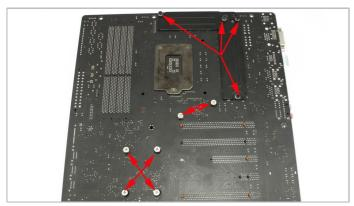
5. With one hand on the block, turn the board back over and refit the ten original screws. You should gradually tighten them in turn so even pressure is applied.
