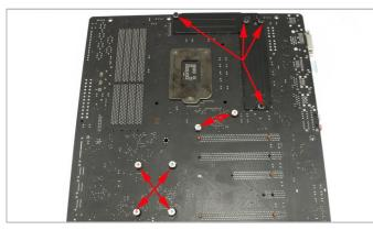
1. Turn the board over and remove the ten screws highlighted above. Keep these to one side, they will be needed in step 5.
