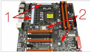
**3.** Place thermal pads on the positions marked 1 and apply a thin layer of thermal paste on positions marked 2.
