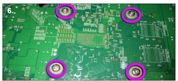
**6**. Finally use the 4 screws and 4 washers to attach the waterblock. It is best to start by screwing in all 4 screws loosely. When you are happy with the position of the block gradually tighten each of the screws. It is important not to overtighten the screws as this could damage the CPU.
