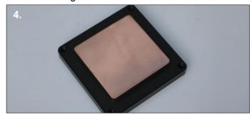
**4.** Remove the protective tape from the waterblock's copper base ready for installation.
