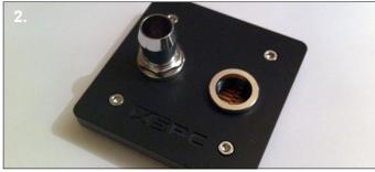
2. If you are using G1/4" barbs/fittings with a long thread you will need to use the supplied rings to avoid blocking the flow.
