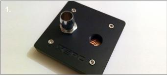
**1**. Screw the barbs into the G1/4" ports using an adjustable spanner. Make sure the o-rings are fully compressed.
