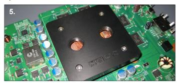
**5**. Place the waterblock over the CPU, making sure the holes on the board line up with the edges of the waterblock. With one hand on the waterblock carefully turn the board upside down.
