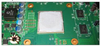
**3**. Clean the CPU to remove any residue left from the old thermal paste. Now apply fresh thermal paste to the CPU core.
