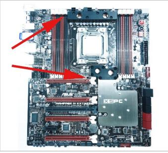
3. Remove the plastic film from the blocks and carefully place the blocks in the positions shown below.
