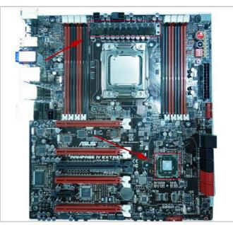
2. Clean the old thermal paste from the chipset. Apply fresh thermal paste to the chipset and place the two thermal pads on the position marked at the top of the board.
