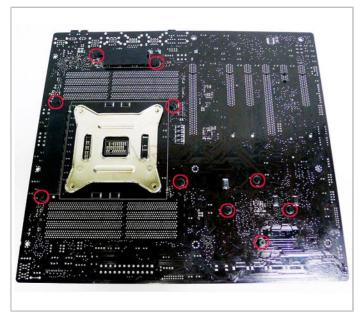
1. Remove the highlighted screws on the back of the motherboard and carefully remove the stock heatsinks.
