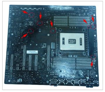
4. Attach the waterblocks using the provided screws. You should be careful to tighten the screws gradually. Over tightening or unevenly tightening the screws could damage the motherboard.
