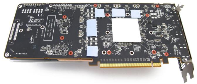
2. Remove the film from both sides of the thermal pads and place them on the location shown above. Place the red washers over the screw holes shown above.
