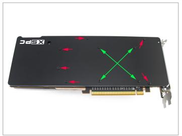
3. Place the backplate onto the card, making sure the front thermal pads and washers stay in place. Now attach the backplate, starting with the four screws marked in green. Do not over tighten the screws as this may bend the card and cause permanent damage.
