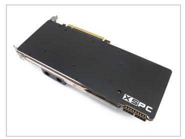
**4**. The card is now ready for use. When you first boot it is advisable to use monitoring software to check the core temperature. If the temperature is high you will need to remount the block.
