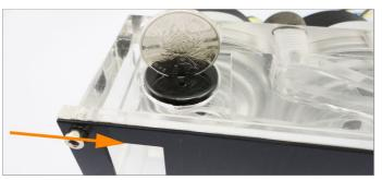
7. The fill cap can be removed using a small coin and turning the cap anti-clockwise. With the fill cap removed fill the reservoir with coolant until it reaches just above the top of the coolant level window. You will have to keep topping up the reservoir as the air bleeds from the loop.
