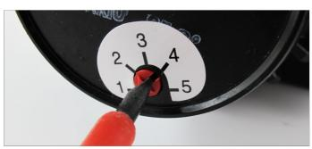
8. The dial on the back of the pump can be used to set the pump speed. 5 being full power and 1 being the lowest noise level. The speed setting on each pump should be matched.
