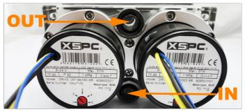
6. Attach your chosen barbs/fittings to the G1/4" inlet and outlet ports. Now attach the tubing and clips.
