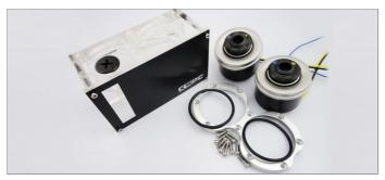
**1**.If you are using a complete D5 pump, first turn the screw ring anti-clockwise to remove the front of the D5 pump. You should also remove the o-ring.
