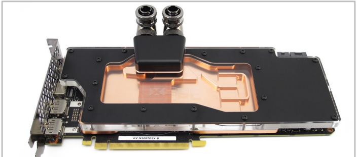
11. Do not over tighten the screws as this may bend the card and cause permanent damage. The card is now ready for use. When you first boot it is advisable to use software to check the core temperature. If the temperature is high you will need to remount the block.
