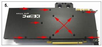
**5**. Place the backplate on the back of the card and attach it using the black M3 screws. You should start with the four screws behind the GPU.
