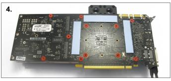
**4**. Flip the card over, making sure the front thermal pads stay in place. Now remove the tape from both sides of the rear thermal pads and place them on the positions shown above. Place the red washers over the screw holes shown above.
