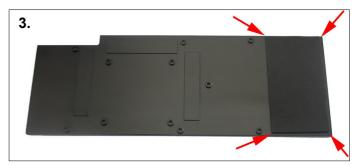
**3.** Stick the pad on the position shown above. The pad is needed to avoid possible shorting if the backplate was accidentally forced against the card.
