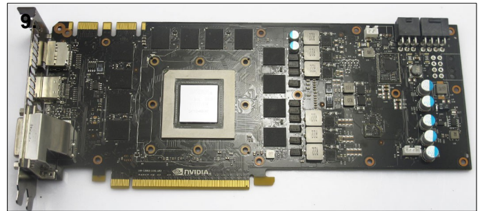
9. Clean the thermal paste from the GPU core and remove any residue left from the thermal pads.
