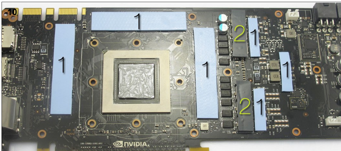
10. Remove the tape from both sides of the thermal pads. Place the blue pads on the positions marked 1 and the grey pads on positions marked 2. Next apply thermal paste to the GPU core.
