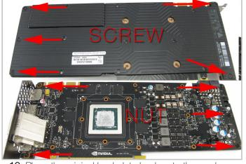
10. Place the original backplate back onto the card. Now use 5 of the original backplate screws and the 5 provided nuts to attach the backplate to the card. This must be done before the block is fitted.
