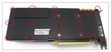
7. Now turn the card on its back and remove the 17 screws highlighted above.
