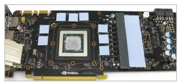
11. Remove the tape from both sides of the thermal pads. Place the blue and grey pads on the ten positions shown above and finally apply thermal paste to the GPU core.
