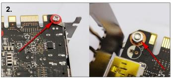
**2**. Use an M3 screw and nut to secure the PCI backplate. Now carefully place the waterblock onto the card and line up the screw holes.
