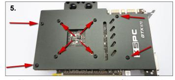
**5**. Place the backplate on the back of the card and attach it using the black M3 screws.
