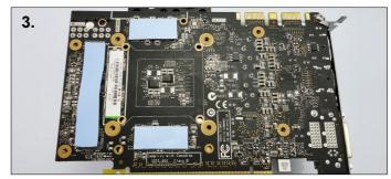
**3.** Flip the card over, making sure the thermal pads stay in place. Remove the tape from both sides of the thermal pads and place them on the positions shown above.
