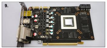
**9.** Clean the thermal paste from the GPU core, and remove any residue left from the thermal pad.
