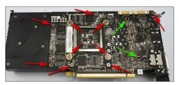
**7.** Turn the card on its back. Remove the 10 screws highlighted in red, and the two clips highlighted in green.
