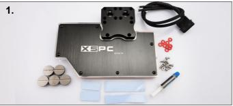
1. The waterblock is designed for SLI setups, so you can fit the G1/4" fittings to multiple sides of the block. Decide which configuration is best for your system.
