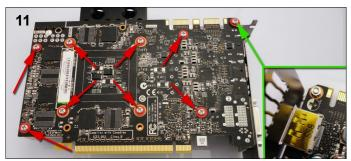
11. First attach the M3 screw marked in green. You will need to use a nut on the other side of the card. Now carefully place the waterblock onto the card and line up the screw holes. Flip it over, making sure the thermal pads stay in place. Finally attach the block to the card using eight M3 screws and washers. You should start with the four screws behind the GPU.
