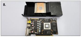
**8**. Turn the card back over and carefully remove the heatsinks and fan. Now the card and heatsinks are separated, detach the fan power cable from the fan header.
