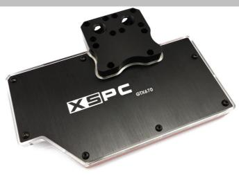
**Note:** This waterblock is only suitable for reference design GTX670 cards. If you are unsure if your card if a reference design GTX670 contact us prior to installation to make sure. **Due to the weight of the block we advise caution when moving your PC.**
