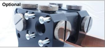
If you are using cards in SLI you can use the optional SLI flow connector to bridge the two cards. This should be done after step 12.
