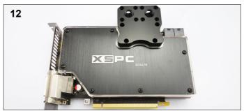
**12**. Do not over tighten the screws as this may bend the card and cause permanent damage. The card is now ready for use. When you first boot it is advisable to use ATItool or other monitoring software to check the core temperature. If the temperature is high you will need to remount the block.
