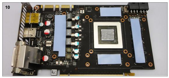
**10**. Remove the tape from both sides of the thermal pads. Place the four blue pads on the positions shown above. Next apply thermal paste to the GPU core.
