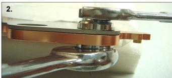
**2.** IMPORTANT: When you install the G1/4" fittings or plugs in steps 2,3 you will need a second wrench on the reverse side of the bulkhead fitting to make sure it doesn't unscrew.
