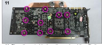
**11.** Place the waterblock on the card and then filp it over to line up the screw holes, making sure the thermal pads stay in place. Now use 10 screws and washers to attach the waterblock to the card. Do not over tighten the screws as this may bend the card and cause permanent damage.
