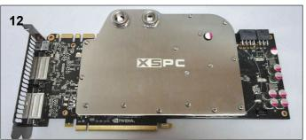
**12**. The card is now ready for use. When you first boot it is advisable to use ATItool or other software to check the core temperature. If the temperature is high you will need to remount the block.
