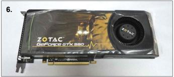
**6**. Before handing the card you should take precautions to avoid static damage. Remove the GTX580 card from the box ready for installation.
