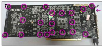
**7.** Remove the two screws on the bracket next to the DVI ports. Now turn the card on its back and remove the 20 screws highlighted above.
