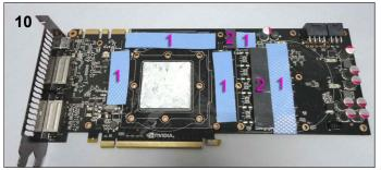
**10**. Remove the tape from both sides of the thermal pads. Place the blue pads on positions marked 1 and grey pads on positions marked 2. Next apply thermal paste to the GPU core.
