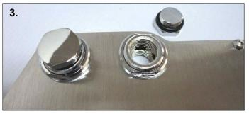
**3**. Use the provided plugs to block the unused G1/4" ports. Make sure the o-rings are fully compressed.
