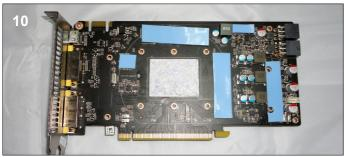
**10**. Remove the tape from both sides of the thermal pads and place them on the 5 locations shown above. Next, apply thermal paste to the GPU core.
