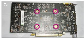
7. Remove the four screws highlighted above.
