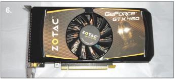
**6**. Before handing the card you should take precautions to avoid static damage. Remove the GTX460 card from the box ready for installation.
