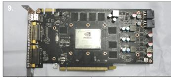
**9.** Clean the thermal paste from the GPU core ready for installation.
