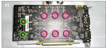
**11.** Place the waterblock on the card and then filp it over and line up the screw holes. Make sure the thermal pads stay in place. Now use six 6mm screws and washers around the GPU core and two 8mm screws behind the VRM part. Do not over tighten the screws as this may bend the card and cause permanent damage.
