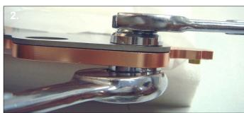
2. IMPORTANT: When you install the G1/4" fittings or plugs in steps 2,3 you will need a second wrench on the reverse side of the bulkhead fitting to make sure it doesn't unscrew.
