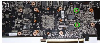
**11.** With the copper side of the waterblock facing up, place the card over the block and line up the screw holes. Make sure the thermal pads have stayed in place and lightly screw two screws with washers into the block through the holes highlighted above and replace the nvidia backplate.
