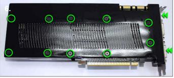
**6.** When handing the card you should take precautions to avoid static damage. Turn the card on its back and remove the 10 screws on the backplate highlighted above. Also remove the two screws near the DVI ports.
