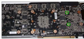
**7.** Carefully remove the nvidia backplate and unscrew the two screws highlighted above.
