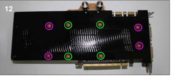
**12**. Finally replace the nvidia backplate and use the 8 provided screws and washers to secure the waterblock to the card. It is best to start with the 4 screws around the GPU to apply the correct pressure to the core. Do not over tighten the screws as this may bend the card and cause damage.
