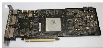
**9.** Clean the thermal paste from the GPU core ready for installation. Remove any residue left from the thermal pads.
