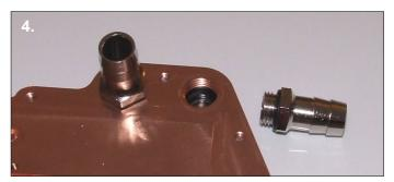
**4.** Attach the barbs to your chosen ports using an adjustable spanner. Make sure the o-rings are fully compressed.
