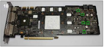
**10**. Remove the tape from both sides of the thermal pads and place them on the locations marked in the photo above. Next apply thermal paste to the memory chips, chipset and the GPU core.
