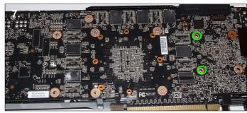
**7.** Carefully remove the nvidia backplate and unscrew the two screws highlighted above.
