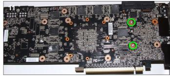
**11.** With the copper side of the waterblock facing up, place the card over the block and line up the screw holes. Make sure the thermal pads have stayed in place and lightly screw two screws with washers into the block through the holes highlighted above.
