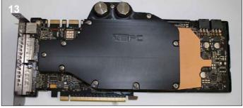
**13.** The card is now ready for use. When you first boot it is advisable to use ATItool or other software to check the core temperature. If the temperature is high you will need to remount the block.
