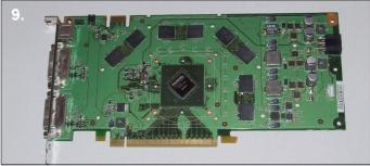
**9.** Clean the thermal paste from the GPU core ready for installation. Remove any residue left from the thermal pads.
