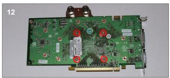
**12**. Finally use the 11 provided screws and washers to attach the waterblock to the card. It is best to start with the 4 screws around the GPU to apply the correct pressure to the core. Do not over tighten the screws as this may bend the card.
