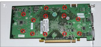
**7.** Turn the card on its back and remove the 12 screws highlighted above.
