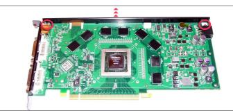
**9.** Unscrew the two screws highlighted above and remove the black aluminium bar. Clean the thermal paste from the GPU core ready for installation. When using thermal pads remember to remove the tape from both sides.
