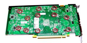
**7.** Turn the card on its back and remove the 12 screws highlighted above.
