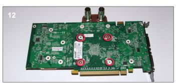
**12**. Finally use the 11 provided screws and washers to attach the waterblock to the card. It is best to start with the 4 screws around the GPU to apply the correct pressure to the core. Do not over tighten the screws as this may bend the card.
