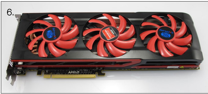
6. Before handling the card you should take precautions to avoid static damage. Remove the 7990 card from the box ready for installation.
