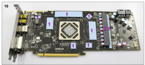
**10**. Remove the tape from both sides of the thermal pads. Place the blue pads on positions marked 1 and the grey pad in the position marked 2. Next apply thermal paste to the GPU core.
