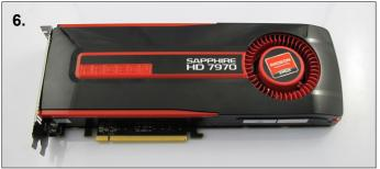
**6**. Before handing the card you should take precautions to avoid static damage. Remove the 7970 card from the box ready for installation.
