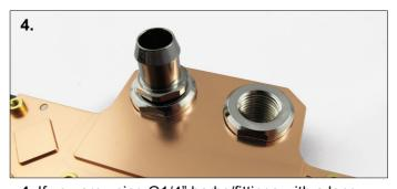
**4.** If you are using G1/4" barbs/fittings with a long thread you will need to use the supplied rings to avoid blocking the flow. Attach the barbs to your chosen ports using an adjustable spanner. Make sure the o-rings are compressed.
