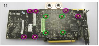
**11.** Place the waterblock on the card and then filp it over to line up the screw holes. Making sure the thermal pads stay in place. Now carefully attach the block to the card, starting with the four holes behind the GPU (marked in green). Next attach the six screws marked in pink.
