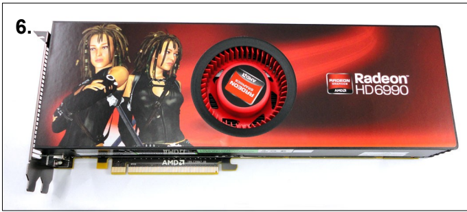
6. Before handing the card you should take precautions to avoid static damage. Remove the 6990 card from the box ready for installation.
