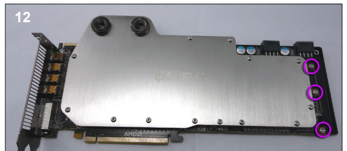
12. Fit the M3 nuts over the screws on the right of the card to secure the backplate. The card is now ready for use. When you first boot it is advisable to use ATITool or other software to check the core temperature. If the temperature is high you will need to remount the block.
