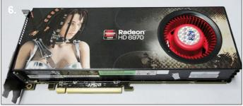
**6**. Before handing the card you should take precautions to avoid static damage. Remove the 6970 card from the box ready for installation.
