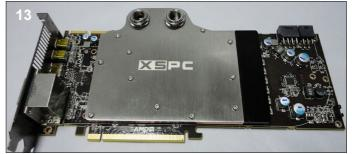
**13.** The card is now ready for use. When you first boot it is advisable to use ATItool, GPU-Z or other software to check the core temperature. If the temperature is high you will need to remount the block.
