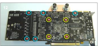
**12**. Finally use the 9 provided screws and washers to attach the waterblock to the card. It is best to start with the 4 screws around the GPU to apply the correct pressure to the core. Do not over tighten the screws as this may bend the card and cause permanent damage.
