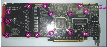
**7.** Remove the two screws on the bracket next to the DVI ports. Now turn the card on its back and remove the 15 screws highlighted above.
