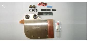
**1**. The waterblock is designed for crossfire setups so you can fit the G1/4" fittings to either side of the block. Decide which configuration is best for your system.
