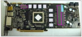
**10**. Remove the tape from both sides of the thermal pads. Place the 3 black pads locations highlighted in purple and the blue thermal pad on the location highlighted in green. Next apply thermal paste to the memory chips and the GPU core.
