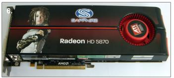
**6**. Before handing the card you should take precautions to avoid static damage. Remove the 5870 card from the box ready for installation.
