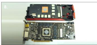
**8**. Turn the card back over and carefully remove the heatsink and fan. Now the card and heatsink are separated detach the fan power cable from the fan header.
