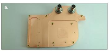
**5**. The block is now ready to be connected to the other watercooling components for leak testing.
