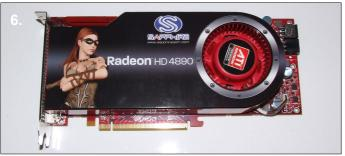
**6**. Before handing the card you should take precautions to avoid static damage. Remove the 4890 card from the box ready for installation.
