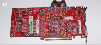
**12**. Finally use the 10 provided screws and washers to attach the waterblock to the card. It is best to start with the 4 screws around the GPU to apply the correct pressure to the core. Do not over tighten the screws as this may bend the card and cause permanent damage.
