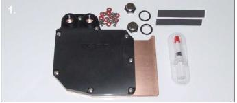
**1**. The waterblock is designed for crossfire setups so you can fit the G1/4" fittings to either side of the block. Decide which configuration is best for your system.
