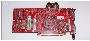
**11.** With the copper side of the waterblock facing up place the card over the block and line up the screw holes. Make sure the thermal pads stay in place.
