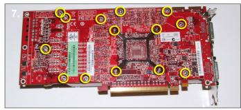
**7.** Turn the card on its back and remove the 14 screws highlighted above.
