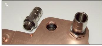
**4.** Attach the barbs to your chosen ports using an adjustable spanner. Make sure the o-rings are fully compressed.
