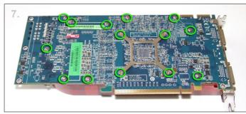
**7.** Turn the card on its back and remove the 14 screws highlighted above.
