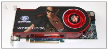
**6**. Before handing the card you should take precautions to avoid static damage. Remove the 4870 card from the box ready for installation.
