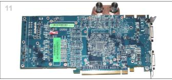
**11.** With the copper side of the waterblock facing up place the card over the block and line up the screw holes.
