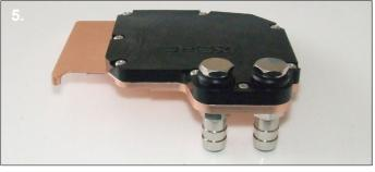
**5**. The block is now ready to be connected to the other watercooling components for leak testing.
