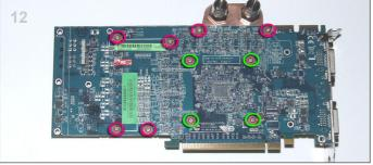
**12**. Finally use the 10 provided screws and washers to attach the waterblock to the card. It is best to start with the 4 screws around the GPU to apply the correct pressure to the core. Do not over tighten the screws as this may bend the card.
