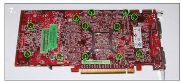
**7.** Turn the card on its back and remove the 12 screws highlighted above.
