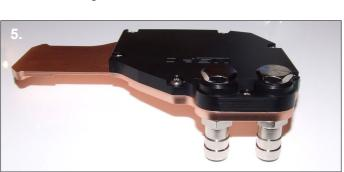
**5**. The block is now ready to be connected to the other watercooling components for leak testing.
