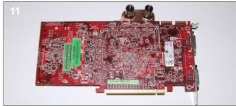
**11.** With the copper side of the waterblock facing up place the card over the block and line up the screw holes.
