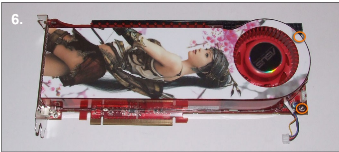
6. Remove the two screws to the right of the fan and unplug the fan power cable from the fan header.
