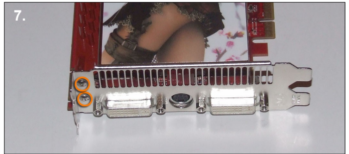
7. Unscrew the two screws on the card plate.
