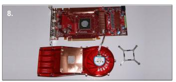
**8**. Turn the card back over to remove the heatsink and fan.
