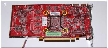
**7.** Turn the card on its back and remove the 4 screws on the backplate.
