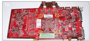
**13.** Finally use the 9 provided screws to attach the waterblock to the card. It is best to start with the 4 screws around the GPU to apply the correct pressure to the core. Do not over tighten the screws as this may bend the card.
