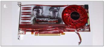
**6**. Before handing the card you should take precautions to avoid static damage. Remove the 3870 card from the box and unplug the fan power cable from the fan header.
