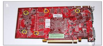
**9.** On the reverse of the card remove the 5 remaining screws.
