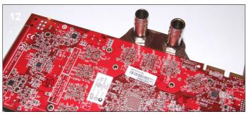
**12**. With the copper side of the waterblock facing up place the card over the block and line up the screw holes.
