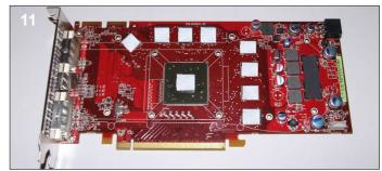
**11.** Remove the tape from both sides of the large thermal pad and place it on the mosfets to the right of the card. Next apply thermal paste to the memory chips and GPU core.
