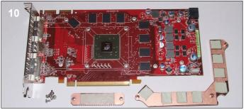
**10**. Carefully apply pressure to take off the two heatsinks and then clean the old thermal paste from the GPU core.
