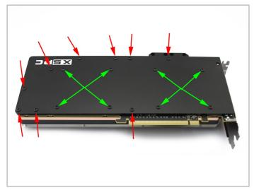
3. Fit the backplate with the provided screws. It's best to fit the screws marked in green first and always tighten each screw gradually. Do not over tighten the screws as this may bend the card and cause permanent damage.
