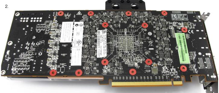
2. Flip the card over - making sure the front thermal pads stay in place. Place the red washers over the screw holes shown above.
