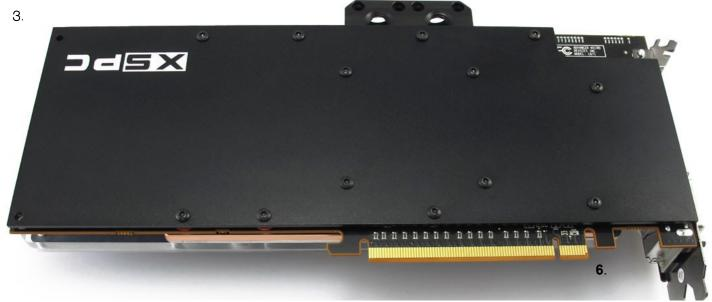
3. Place the backplate on the back of the card and attach it using the black M3 screws. You should start with the four screws behind the GPU. Do not over tighten the screws as this may bend the card and cause permanent damage.
