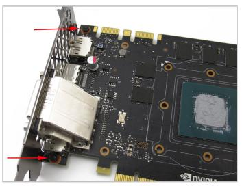
2. Reattach the PCI plate using two M2.5 screws and nuts.
