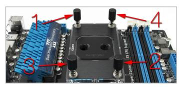
6. Place a nut onto each post and gradually tighten them. You should tighten each nut in stages. e.g. 1,2,3,4,1,2,3,4,1,2,3,4, until each nut is fully tightened.
