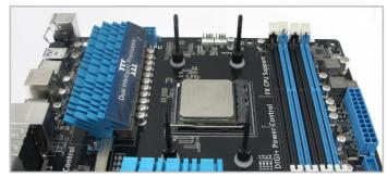
3. Place a nylon washer over the short end of each post and screw it into each of the four holes around the socket.
