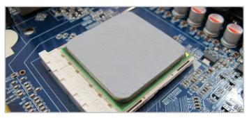
2. Apply a thin layer of thermal paste to the CPUs heat spreader.
