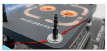
4. Place a plastic washer and metal washer over each of the four posts. If using socket AM4 use two plastic washers and one metal washer.
