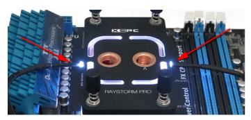
7. Push the LEDs into either side of the waterblock.
