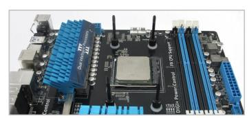
3. Place a nylon washer over the short end of each post and screw it into each of the four holes around the socket.
