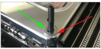
3. Place a plastic washer and metal washer over each of the four posts.
