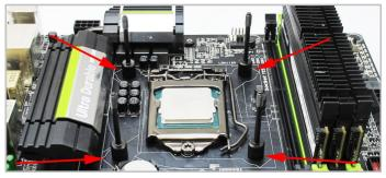
4. Screw the short end of the M3 posts into each of the four holes around the socket.
