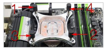
6. Place a nut onto each post and gradually tighten them. You should tighten each nut in stages. e.g. 1,2,3,4,1,2,3,4,1,2,3,4, until each nut is fully tightened.
