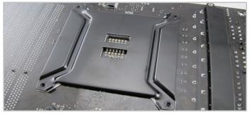
3. Make sure the 4 screw threads on the backplate line up with the holes on the motherboard. Apply pressure to secure the backplate.
