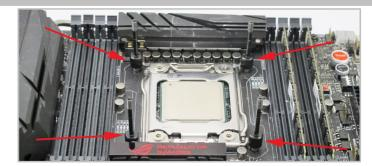
2. Screw the short end of the M4 post into each of the four holes around the socket.
