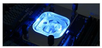
8. The block is now ready to use. When you first boot it is advisable to use software to check the core temperature. If the temperature is high you will need to remount the block.
