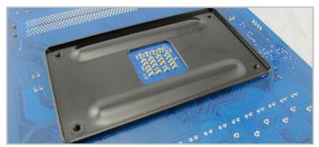
2. If the backplate is loose, place it back in its correct position. Make sure the 4 screw threads on the backplate line up with the holes on the motherboard.
