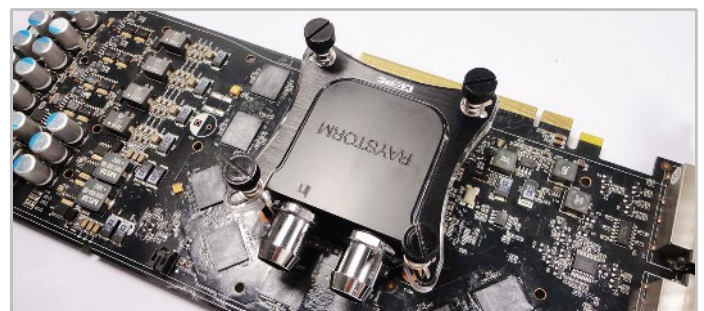
8. The card is now ready for use. When you first boot it is advisable to use ATITool or other software to check the core temperature. If the temperature is high you will need to remount the block.
