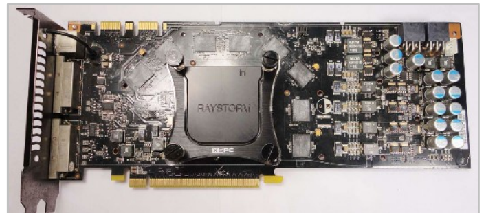
4. With the spring and washers in place, put a screw through the mounting plate and the hole on the card. Repeat this for each thumb screw.
