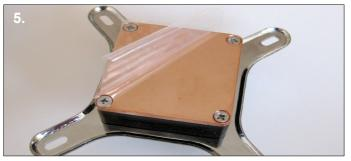
**5**. Remove the plastic film from the base of the waterblock and apply thermal paste to the CPU.
