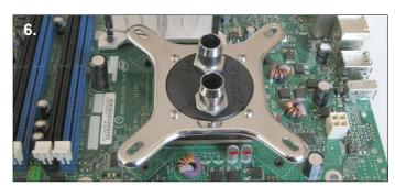
**6**. Place the waterblock onto the CPU and line-up the mounting plate with the holes on the motherboard.
