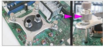
**8**. Use the lower knurled nut to partly compress the spring and adjust the pressure on the CPU. Make sure to apply equal pressure to each spring.
