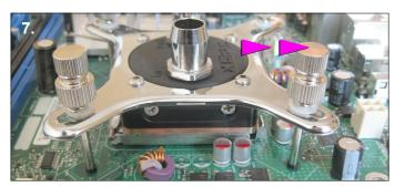
7. Place each of the bolts through the mounting plate and loosely screw into the backplate using the top knurled section. When all 4 are fitted tighten each bolt.
