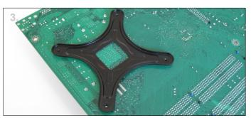
**3**. Place the backplate on the back of the motherboard and line up the holes. Apply pressure to secure.
