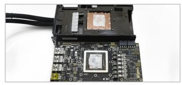
9. Carefully remove the heat sink and detach the power cable from the power header.
