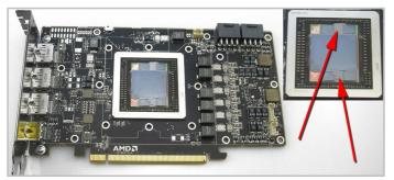
10. Clean the thermal paste from the GPU core and memory stacks with a soft cloth. Do not attempt to clean any paste left between the core and memory stacks, as this can cause damage.
