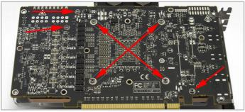
12. Place the waterblock on the card to line up the screw holes and then flip it over (make sure the thermal pads stay in place). Fit the original screws to the positions marked above. Do not over tighten the screws as this may bend the card and cause permanent damage.
