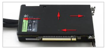
7. Turn the card on its back and remove the 4 screws highlighted above and remove the backplate.
