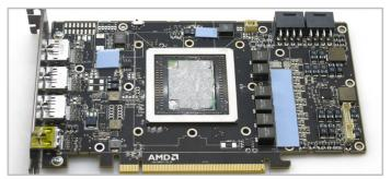
11. Remove the tape from both sides of the thermal pads and place them on the three positions shown above. Now apply thermal paste to the GPU core and memory stacks.
