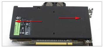
13. Refit the backplate and attach it using the two screws shown above.
