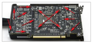
**8**. With the backplate removed, unscrew the 13 screws highlighted above.
