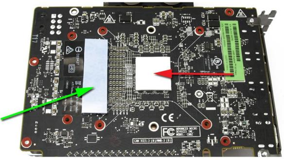
2. Flip the card over (make sure the front thermal pads stay in place). Place the red washers over the screw holes shown above. Now remove the protective film from both sides of the thermal pads. Place the 1.5mm pad on the position marked in red and the 1mm pad on the position marked in green.
