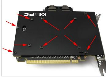
3. Fit the backplate with the provided screws. Do not over tighten the screws as this may bend the card and cause permanent damage.
