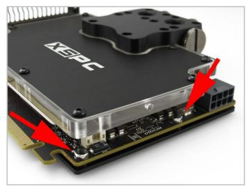
4. Finally turn the card over and secure the screws shown above with the provided nuts.
