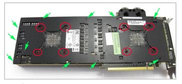
11. Place the waterblock on the card to line up the screw holes and then flip it over, making sure the thermal pads stay in place. First fit the M3 screws and washers (marked in red). Finally fit the original backplate and use the countersink screws to attach it (marked in green). You should gradually tighten each screw to apply even pressure..
