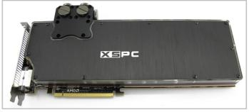
12. Do not over tighten the screws as this may bend the card and cause permanent damage. The card is now ready for use. When you first boot it is advisable to use software to check the core temperature. If the temperature is high you will need to remount the block.
