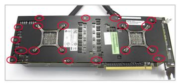
7. Now turn the card on its back and remove the 19 screws highlighted above.
