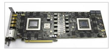
**9.** Clean the thermal paste from the GPU cores and remove any residue left from the thermal pads.
