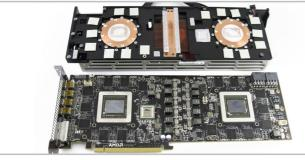
**8**. Turn the card back over and carefully remove the heat sink and fan. Now the card and heat sink are separated detach the fan power cable from the fan header.
