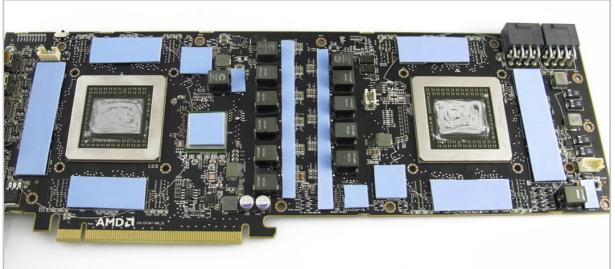
10. Remove the tape from both sides of the thermal pads. Place the blue pads on the fourteen positions shown above and finally apply thermal paste to the GPU cores.
