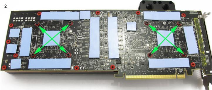
2. Flip the card over, making sure the front thermal pads stay in place. Place the red washers over the screw holes shown above and fit the eight crosshead screws on the positions marked in green. Now remove the protective film from both sides of the thermal pads and place them on the fifteen locations shown above.
