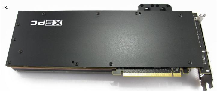
3. Place the backplate on the back of the card and attach it using the allen head screws. Tighten each screw gradually and do not over tighten the screws as this may bend the card and cause permanent damage.
