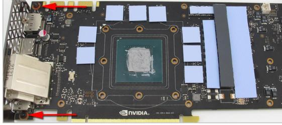
**9**. Remove the tape from both sides of the thermal pads. Place the blue and grey pads on the twelve positions shown above and finally apply thermal paste to the GPU core. Place the waterblock on the card to line up the screw holes and then flip it over (make sure the thermal pads stay in place).
