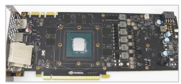
7. Clean the thermal paste from the GPU core and remove any residue left from the thermal pads.
