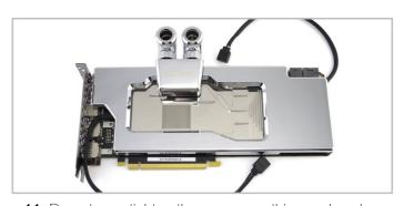
11. Do not over tighten the screws as this may bend the card and cause permanent damage. The card is now ready for use. When you first boot it is advisable to use software to check the core temperature. If the temperature is high you will need to remount the block.
