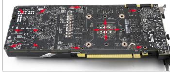
5. Remove the backplate and remove the 14 bolts highlighted above.
