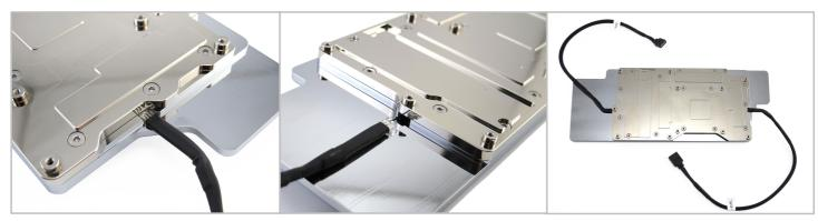
3. The LEDs must be fitted before the block is installed to the card. Simply insert the LEDs into the LED holes on the left and right side of the waterblock. The waterblock is now ready for installation.
