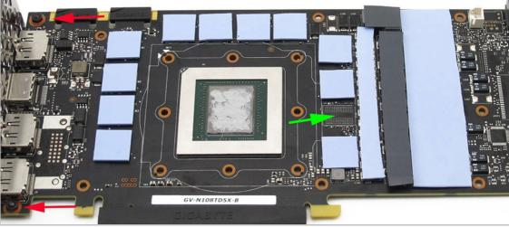
**9**. Remove the tape from both sides of the thermal pads. Place the blue and grey pads on the fifteen positions shown above (sixteen for Titan X Pascal) and finally apply thermal paste to the GPU core. Place the waterblock on the card to line up the screw holes and then flip it over (make sure the thermal pads stay in place).
