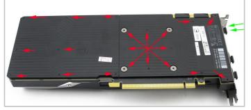
**4**. Turn the card on its back and remove the 22 screws highlighted above.
