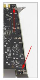
8. Use two of the provided screws and two nuts to secure the I/O bracket. This must be done before the block is fitted.
