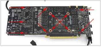
10. Now fit the supplied screws and washers in positions marked red. You should gradually tighten each screw to apply even pressure.
