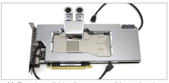
11. Do not over tighten the screws as this may bend the card and cause permanent damage. The card is now ready for use. When you first boot it is advisable to use software to check the core temperature. If the temperature is high you will need to remount the block.
