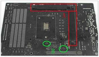
5. With one hand on the block, turn the board back over. Refit four of the original screws on positions marked A and the supplied screws on positions marked B. You should gradually tighten them in turn so even pressure is applied.
