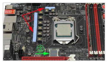
3. Remove the film and place the blue thermal pads on the positions marked 1 and the grey pad on the position marked 2.
