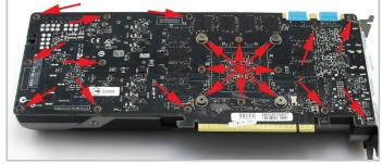
7. Now turn the card on its back and remove the 20 screws highlighted above.
