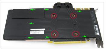
**12.** Place the waterblock on the card to line up the screw holes and then flip it over, making sure the thermal pads stay in place. First fit the M2.5 screws and washers (marked in red). Finally fit the original screws to attach it (marked in green). You should gradually tighten each screw to apply even pressure..
