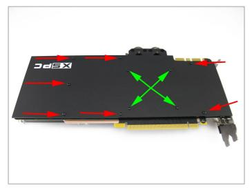
4. Place the backplate onto the card, making sure the front thermal pads and washers stay in place. Now attach the backplate, starting with the four screws marked in green. Do not over tighten the screws as this may bend the card and cause permanent damage.
