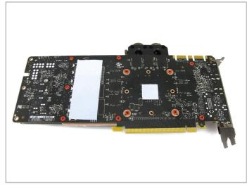
**3.** Remove the film from both sides of the thermal pads and place them in the locations shown above. Place the red washers over the screw holes shown above.
