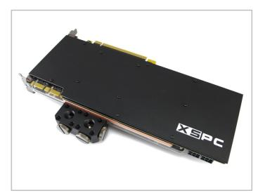
**5**. The card is now ready for use. When you first boot it is advisable to use monitoring software to check the core temperature. If the temperature is high you will need to remount the block.
