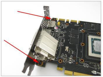
2. Reattach the PCI plate using two M2.5 screws and nuts.
