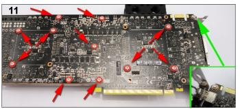
**11.** Place the waterblock on the card to line up the screw holes and then filp it over, making sure the thermal pads stay in place. Now carefully attach the block to the card using twelve M3 screws and washers. The screw marked in green requires an M3 nut attaching on the other side of the card.
