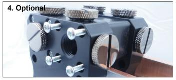
**4.** If you are using cards in SLI you can use the optional SLI flow connector to bridge the two cards. This should be done after step 12.
