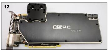
**12**. Do not over tighten the screws as this may bend the card and cause permanent damage. The card is now ready for use. When you first boot it is advisable to use ATItool or other monitoring software to check the core temperature. If the temperature is high you will need to remount the block.
