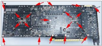
**7.** Now turn the card on its back and remove the 19 screws highlighted above.
