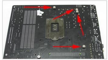
1. Turn the board over and remove the four screws highlighted above. Keep these to one side, they will be needed in step 5.
