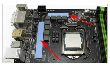
3. Remove the film from both sides and place the blue thermal pads on the positions marked above.
