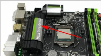
2. Turn the board back over and slowly remove the stock heat sink from the board. You should be careful not to damage any components on the board.
