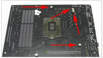
5. With one hand on the blocks, turn the board back over. Refit the four original screws to secure the blocks. You should gradually tighten them in turn so even pressure is applied.
