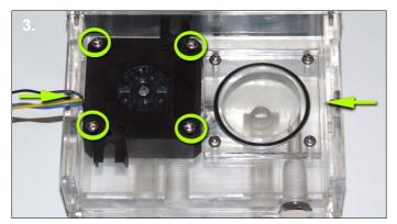
**3**. Place the pump onto the reservoir making sure that the o-ring stays in place. The pump should be orientated so the wires are on the outer sides of the reservoir. Use the 4 long screws to attach the pump to the reservoir, tightening them until the large o-ring is compressed.
