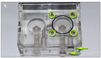
**1**. Turn the reservoir upside down. If you are using two pumps, remove the blanking plate and two G1/4" plugs.
