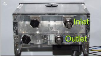
**4.** Repeat stage 3 on the opposite side if you are using two pumps. Now screw the G1/4" fittings to the inlet and outlet making sure the o-rings are compressed. The pump is now ready to be connected to your other watercooling components and leak tested before being fitted into two 5.25" drive bays.
